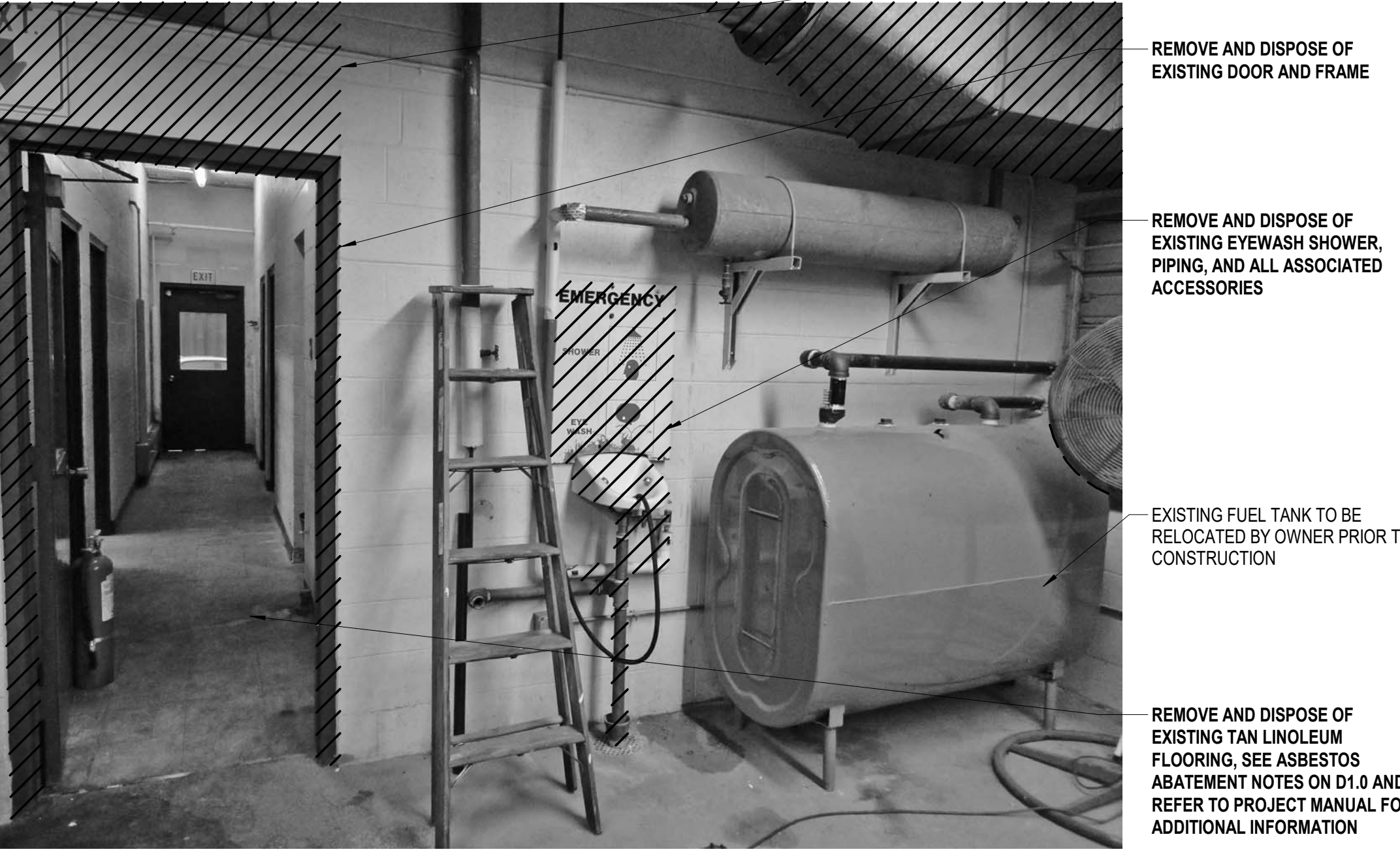
Control Building Eyewash and Door Demolition Detail
