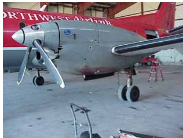
This Saab 340 hit a deer on landing at a Midwest USA airport in April 2000, ripping the engine from its mountings (photo courtesy Northwest Airlines).
